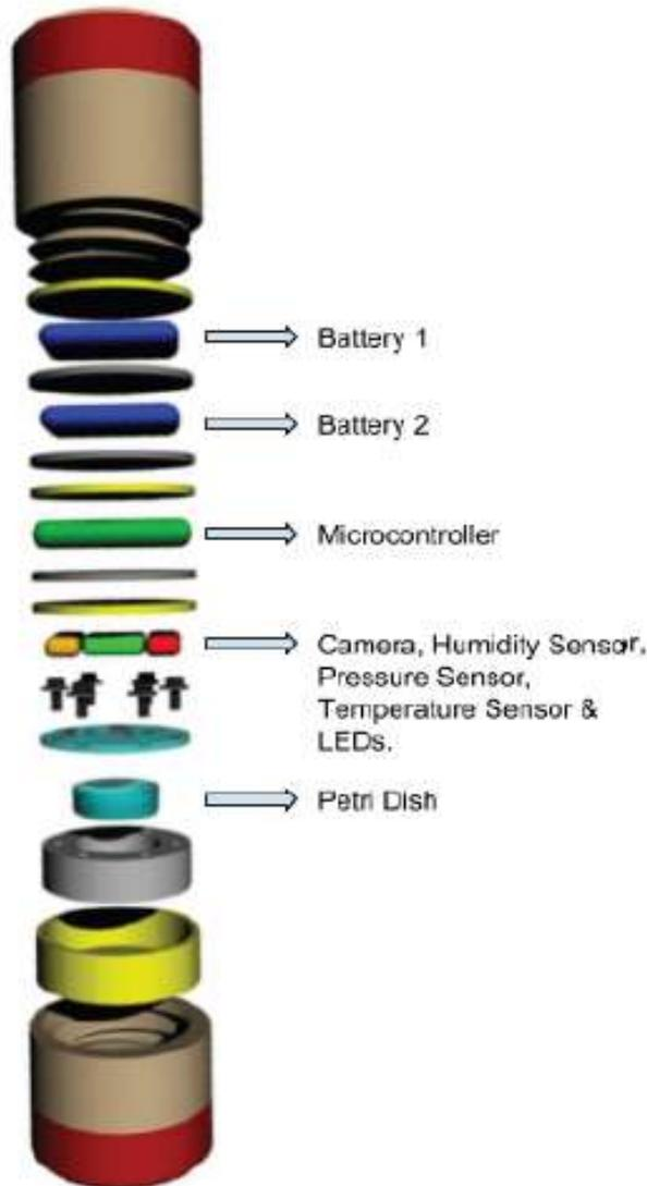
The monitoring system from capsule will be based on a Raspberry Pi Zero specifications. The system will consume between 0.5 - 0.7W and it can work with a USB 5V as power supply. Camera, LEDs and some sensors will be activated every 6 hours so they don't need much energy. Temperature sensor and resistance are the only components that will be active all time. We have an extra power source which will help us if we have an emergency situation.
